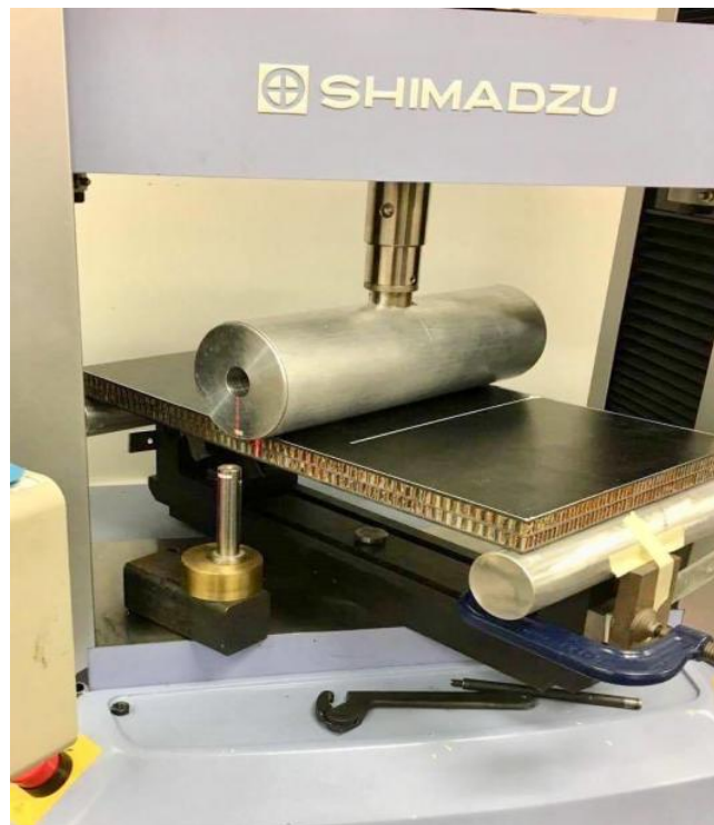
Fig 12: Three-Point Bending Test Assembly
