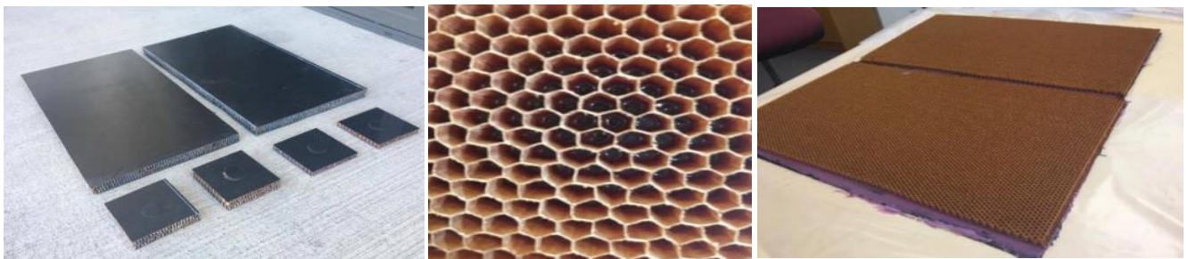
Fig 5 (L to R): Single and Double Core CFRP-Nomex Sandwich Panels, Depiction of Formation of Adhesive Fillets and Bonding of CFRP Skins to Nomex Honeycomb Core
